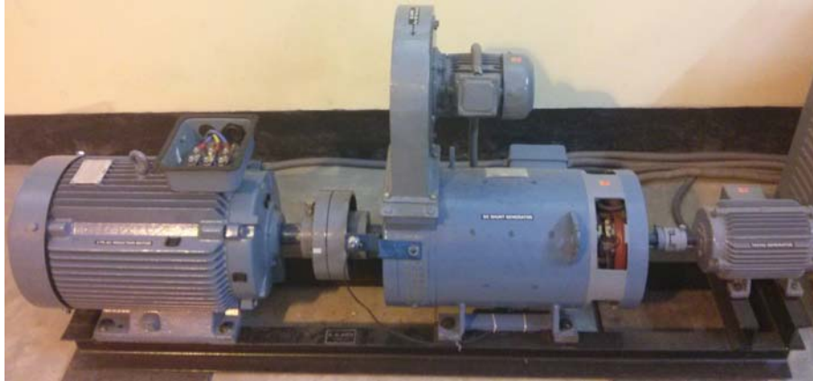
Figure 4.7: The motor-generator experimental setup
